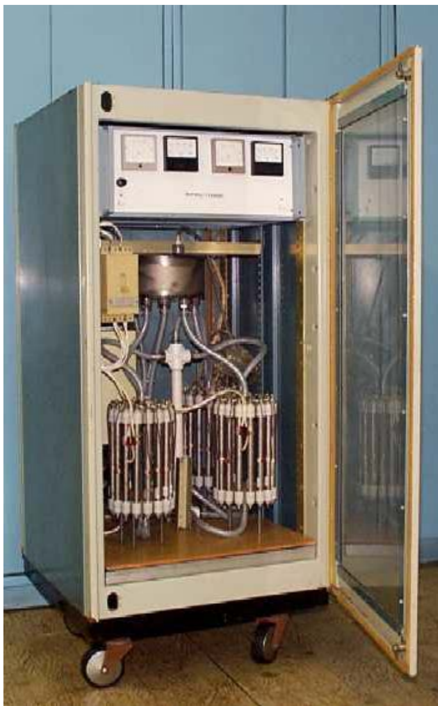
STEL-1000-SK device with productivity of 1000 l/h of anolyte ANK used for silage feed. Two reactors RPE-20 of 20 FEM-3 elements in each reactor are used in the device. Power consumption 2.5 kW. Moscow, 1994. In the period from 1990 to 1994 in STEL-1000-SK device the reactor from two graphite monoblocks in titanium cases was used (right).
