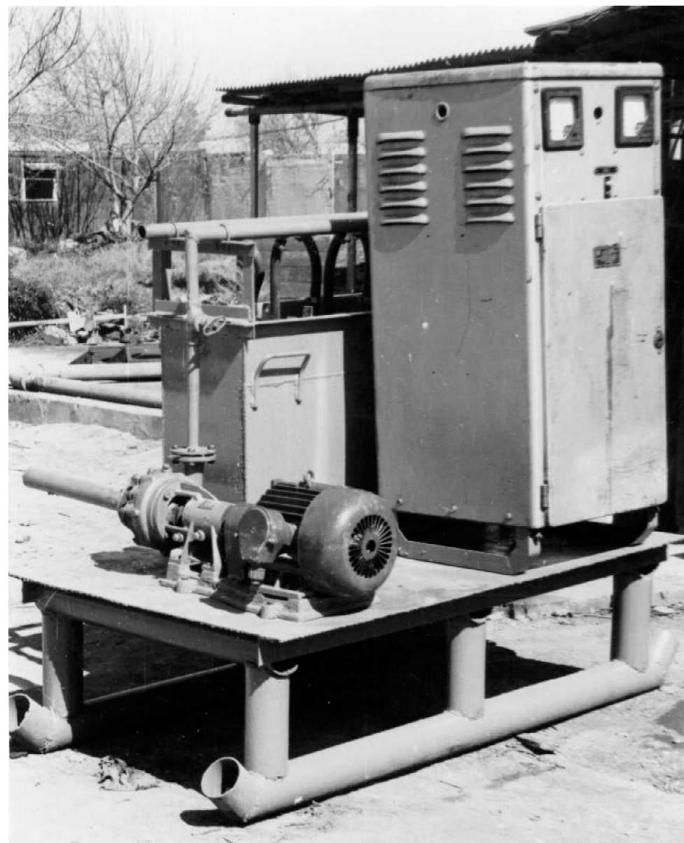
Productivity of individual devices for electrochemical water treatment (UEW) with flat electrodes reached 20 m 3 /h by 1976 (photo right). It helped to use it not only for drill, where activated water – catholyte - was used for preparation of drilling fluids and cooling of diesel engines, but also in the process of oil displacement at edge waterflooding and boundary waterflooding. The photo on the left is one of the places of maintaining of formation pressure at the oil field PO "UZBEKNEFT", 1976.
