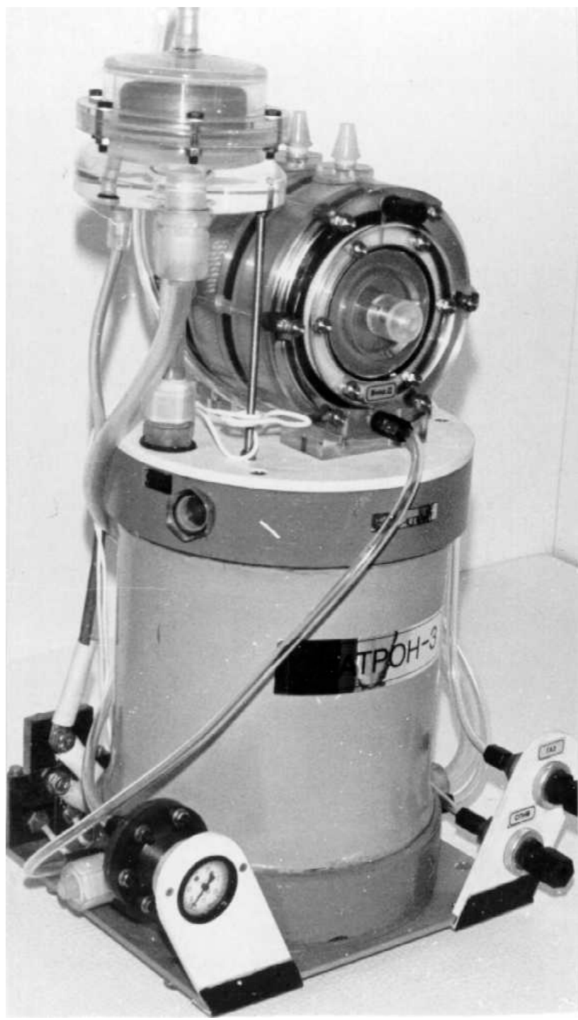
ECATRON-01 device to obtain catholyte and anolyte from drinking water, used in technologies of industrial poultry farming. In the device the electrochemical reactor of ELCA-003 device is used with the cathode in the form of a graphite monoblock with 19 cells. Productivity is 250 l/h, current - up to 100 A, voltage - up to 70 V. Moscow, NPK "ASPECT", 1989
