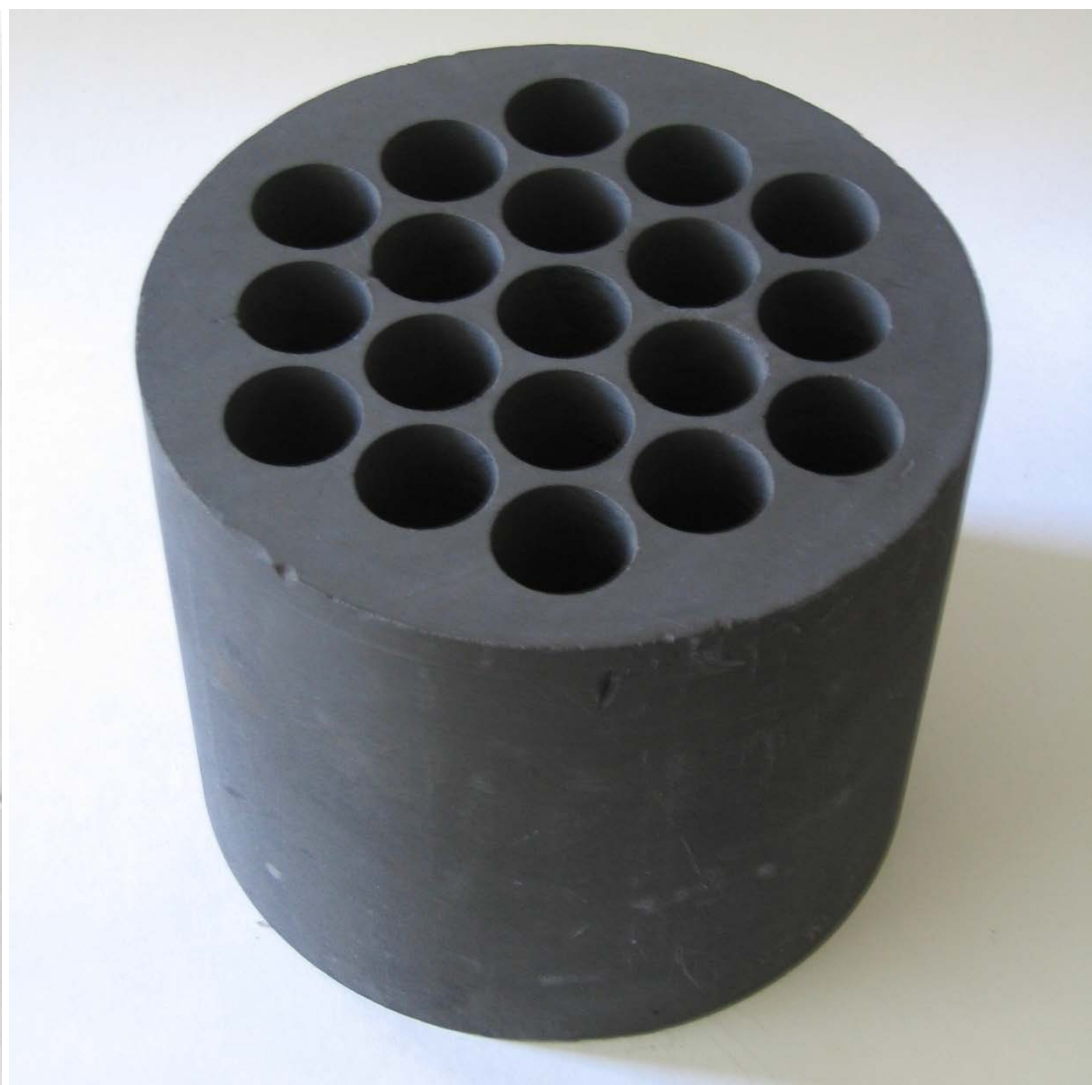
ECATRON-01 device to obtain catholyte and anolyte from drinking water, used in technologies of industrial poultry farming. In the device the electrochemical reactor of ELCA-003 device is used with the cathode in the form of a graphite monoblock with 19 cells. Productivity is 250 l/h, current - up to 100 A, voltage - up to 70 V. Moscow, NPK "ASPECT", 1989
