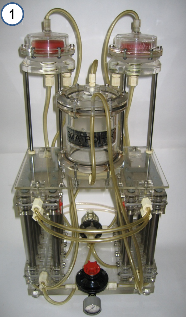
1-experimental model of ECATRON-K device for obtaining gaseous hydrogen chloride as an effective agent for straw saccharification. Manufactured according to requirement specification of professor K.A. Kalunyants. RPE-10L reactors (4) with FEM-1 elements (3) are used in the device for the first time. Moscow, Moscow technological Institute of food industry, 1989.
