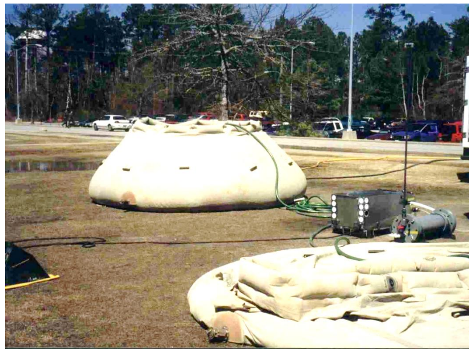
STEL device with FEM-3 elements for US Marines during the field tests on the ground in Atlanta, 1996. FEM-3 elements are mounted in three RPE-S-36 reactors (36 FEM-3 elements in each reactor).
