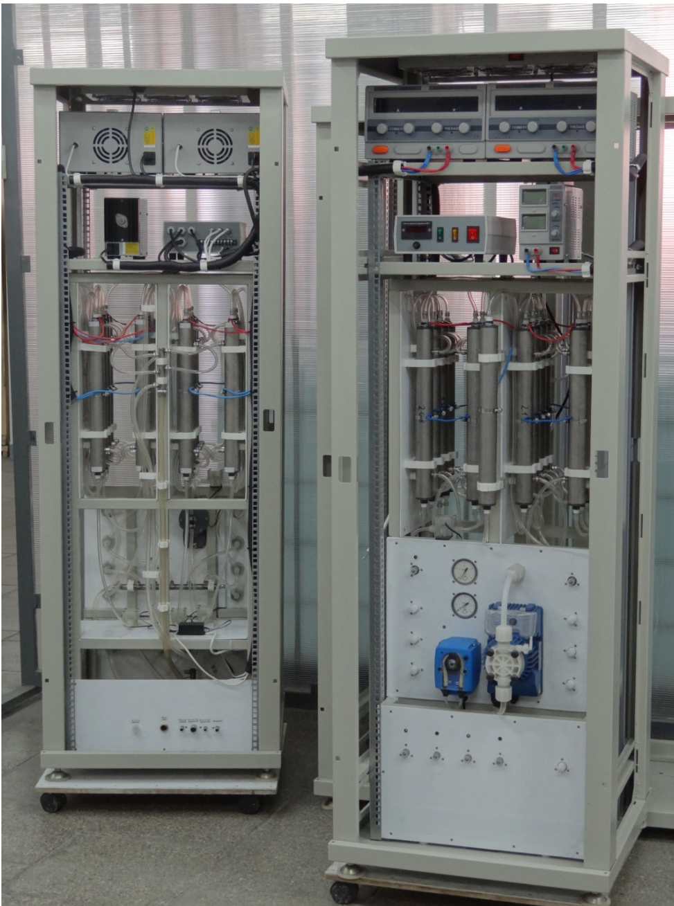
STEL-UNIVERSAL devices with productivity of 500 l/h for anolyte and catholyte. On the right is the model of 2008, on the left - model of 2011 year.
