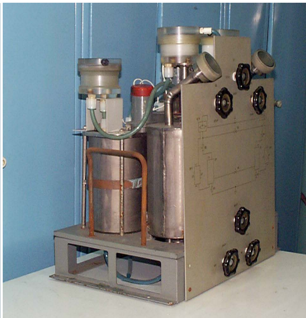
STEL-1000-SK device with productivity of 1000 l/h of anolyte ANK used for silage feed. Two reactors RPE-20 of 20 FEM-3 elements in each reactor are used in the device. Power consumption 2.5 kW. Moscow, 1994. In the period from 1990 to 1994 in STEL-1000-SK device the reactor from two graphite monoblocks in titanium cases was used (right).
