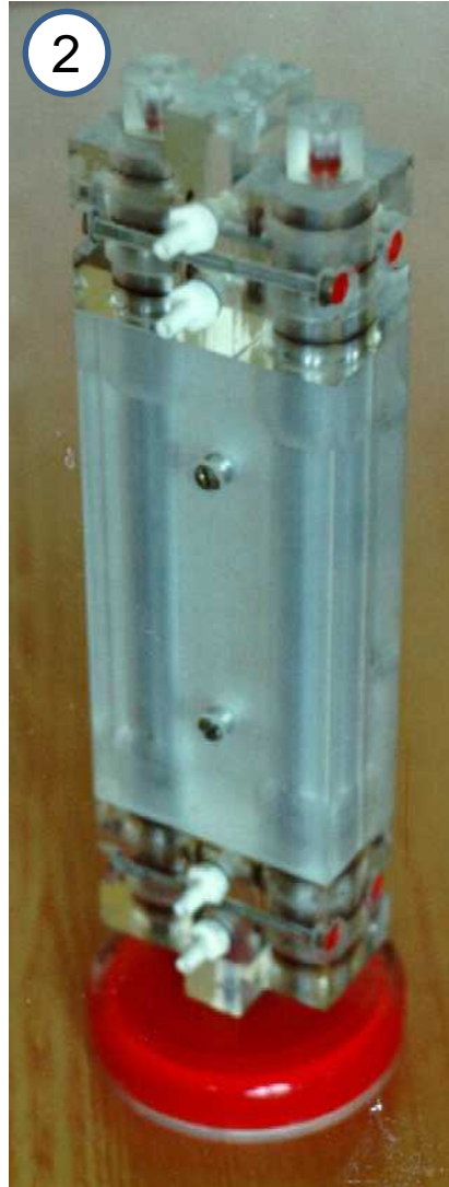
1-experimental model of ECATRON-K device for obtaining gaseous hydrogen chloride as an effective agent for straw saccharification. Manufactured according to requirement specification of professor K.A. Kalunyants. RPE-10L reactors (4) with FEM-1 elements (3) are used in the device for the first time. Moscow, Moscow technological Institute of food industry, 1989.
